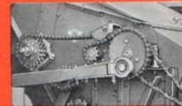
A cylinder speed for every harvesting need. 245 r.p.m. to 1178 r.p.m.
