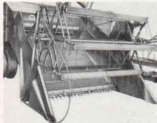
Full width pick-up and swath spreader for windrowed crops.
