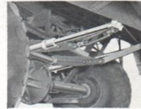
Two hydraulic cylinders smoothly change cutting height.
