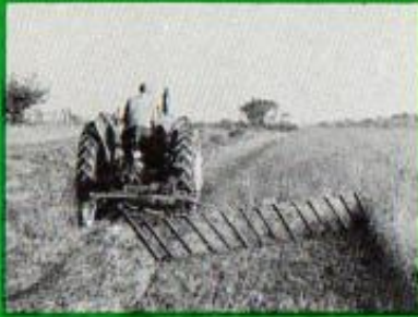
Cockshutt "15AS" Mower equipped with windrower — available for either 6' or 7' cutter bar.
